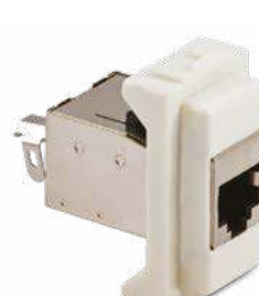
6099 Presa RJ45 plug 8/8cc Cat.6 STP schermata
